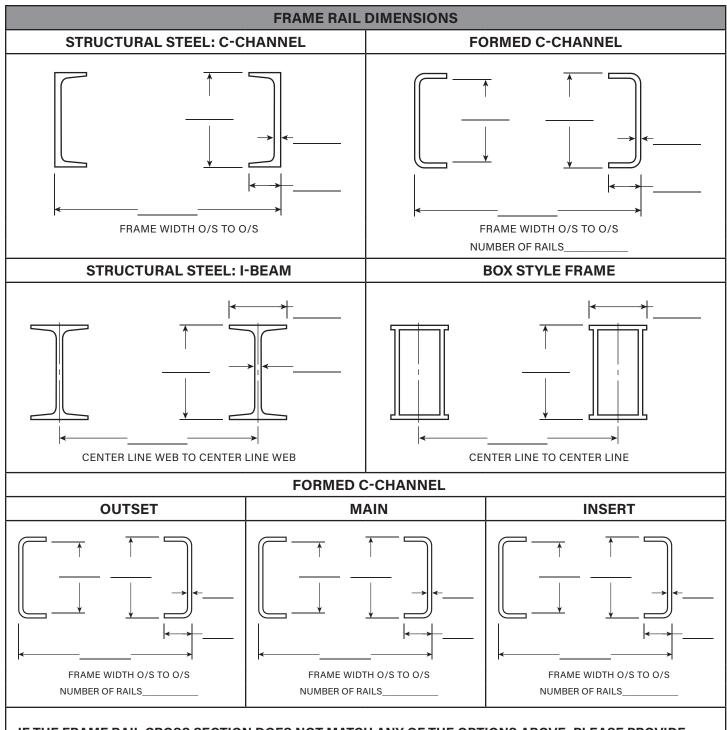
IF THE FRAME RAIL CROSS SECTION DOES NOT MATCH ANY OF THE OPTIONS ABOVE, PLEASE PROVIDE DRAWINGS AND DIMENSIONS WITH APPLICATION FORM.
