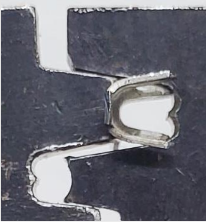
Figure 13 B-form Terminal Crimping
