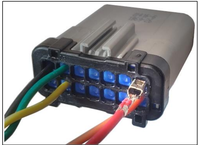
Figure 11 RP1226 Connector Terminal Insertion
