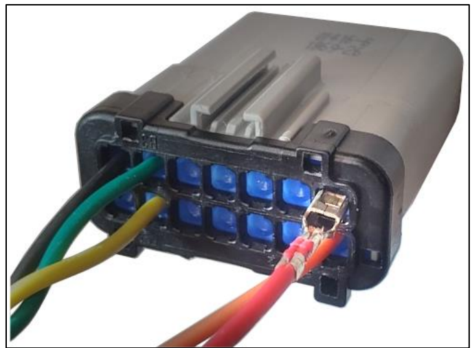
Figure 11 RP1226 Connector Terminal Insertion
