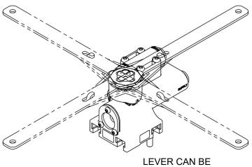
LEVER CAN BE MOUNTED IN ANY ONE OF FOUR POSITIONS
