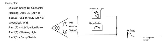
■ **NOTE:** The warning indicator light MUST be a LED type light with a maximum current draw of **30 milliamps**. An incandescent light or any light exceeding a current draw of 30 milliamps will not function properly.
