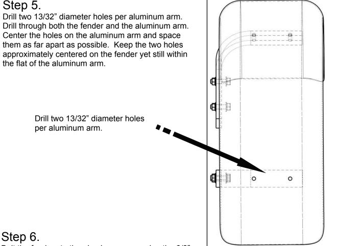
Bolt the fenders to the aluminum arms using the 3/8" Truss Head Bolts and the 3/8" Top Lock Nuts.
