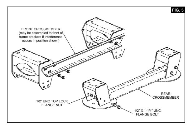
**9.8** Assemble the suspension to the front frame brackets using the provided mounting hardware (See **Fig. 6** for fastener detail)
