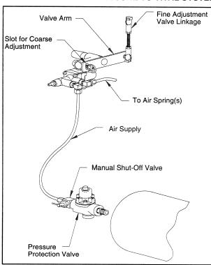
WARNING: LOSS OR APPLICATION OF AIR PRESSURE TO CABMATE WILL CAUSE SUDDEN MOVEMENT OF THE CAB. PRIOR TO INSTALLING OR PERFORMING ANY MAINTENANCE, BLOCK UP THE CABMATE TO PREVENT THE POSSIBILITY OF INJURY.
