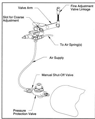
WARNING: LOSS OR APPLICATION OF AIR PRESSURE TO CABMATE WILL CAUSE SUDDEN MOVEMENT OF THE CAB. PRIOR TO INSTALLING OR PERFORMING ANY MAINTENANCE, BLOCK UP THE CABMATE TO PREVENT THE POSSIBILITY OF INJURY.
