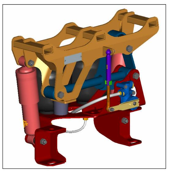
The **CABMATE MODEL KWT2000-A** fits Kenworth T2000 conventionals. It replaces the original cab suspension on trucks manufactured prior to April, 1999.
