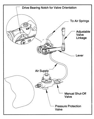
LOSS OR APPLICATION OF AIR PRESSURE TO CABMATE WILL CAUSE SUDDEN MOVEMENT OF THE CAB. PRIOR TO INSTALLING OR PERFORMING MAINTENANCE, BLOCK UP THE CABMATE TO PREVENT THE POSSIBILITY OF INJURY.
