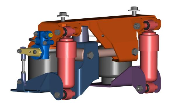
The **CABMATE MODEL NAV80** fits most International S2500, S2600, 8100, 8200, and 8300 Series Conventionals. It replaces the original rear cab mounts (center mount), International Part No. 476979-C1.
