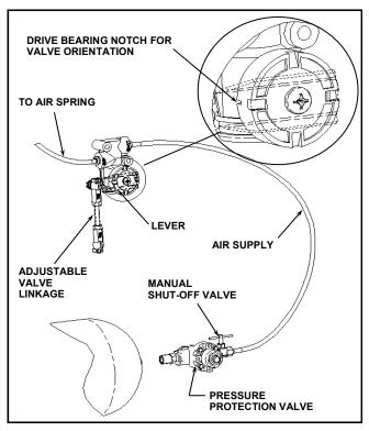
WARNING: LOSS OR APPLICATION OF AIR PRESSURE TO CABMATE WILL CAUSE SUDDEN MOVEMENT OF THE CAB. PRIOR TO INSTALLING OR PERFORMING MAINTENANCE, BLOCK UP THE CABMATE TO PREVENT THE POSSIBILITY OF INJURY.
